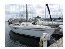
35' 5" LOA LWL 13' 0" 4' 6" Beam Draft (wing keel) Displacement 11,700 lbs **Ballast** 4,400 lbs ~781 ft<sup>2</sup> Sail Area Bridge Clearance 52' 6" 39 gals. Fuel Water 89 gals. 6' 9" 22 gals. Cabin Headroom Waste Universal M35B 4 cyl diesel, 35 HP, 720 Hours Power
