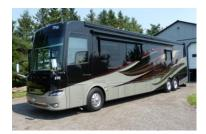
44' 11" Length Width 101.5" Height 12' 11" Interior width 95.5" Fuel 105 U.S. gallons 150 U.S. gallons Water Grey water 65 U.S. gallons Sewage 45 U.S. gallons Propane 22 U.S. Gallons 50.000 btu Furnace Generator 12.5 kW Air Units 3 x15.000 btu Power Cummins 12 ISX Diesel, Allison 4000 MH transmission
