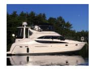
40' LOA 42' 2" Length 14'4" 3' 10" Beam Draft Modified "V" **Hull Type Dead Rise** 10° Fuel 330 U.S. gallons Water 90 U.S. gallons 55 U.S. gallons Waste Weight 29,000 lbs (Dry) Headroom 6'6" Sleeps Twin Cummins 370 Diamond Series ~ 750 hours Power
