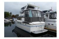
36' 6" 12' 10" Length Beam 3' 2" Draft Fuel 300 gal Water Waste 100 gal 2 tanks 11' 6" 20,400# Clearance Weight Headroom 6'3" Sleeps 7
