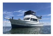
LOA 39' 9" 34' 9" (less pulpit and platform) Hull Length 14' 2" 300 USG/1136L Beam Fuel 3' 8" Draft Water 118 USG/447L Weiaht 22,000# (dry) Waste 35 USG/132L 6' 6" Clearance Headroom 19' (incl sat TV)
