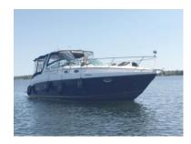
**37' 0"** (w/swim platform) 12' 0" Length **Beam** 35"/24" Draft Weight 14.280 # 235 gallons **Fuel** Water 51 gallons Waste 45 gallons Headroom 6' 10"
