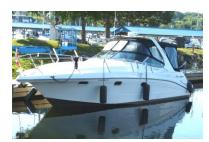
LOA 35' 1" (w/swim platform) Length 33' 5" 11' 9" 3' 3" Beam Draft Fuel 220 gallons Water 45 gallons Waste 30 gallons Weight 12,000 lbs 19° Sleeps 4-5 Deadrise
