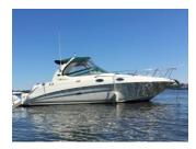
LOA **Hull length** 28' 6" 31' 1" (w/std. ext. swim platform) Weight Beam 9' 5" 8,500 lbs Draft 23/39" Fuel 100 Gallons Water 28 Gallons Waste 28 Gallons
