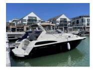
LOA 31' 0" 9' 11" Beam Draft 3' 3" Fuel 103 gallons Water 27 gallons Waste 17 gallons Weight 8,350 lbs (dry) Clearance 8' 10" Deadrise Aft 21° Sleeps 6
