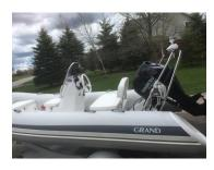
LOA 12' 2" Beam 6' 1" Depth 18" Weight 273 lbs with 30hp motor Seats 5 Power 30hp Tohatsu 4 stroke with electric start
