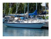
LOA 28' 7" 22' 0" LWL 9' 3" 4' 4" Beam Draft 13 Gallons Fuel 12 Gallons Water Waste 18 Gallons Weight 8.500 lbs
