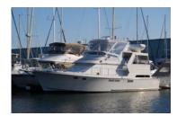
Length 44' 2" LOA 50' 0" 36" 14' 8" Draft Beam Fuel 600 Gallons Water 140 Gallons Waste 60 Gallons Weight 28,000 lbs (dry)
