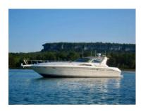
45' 7" (w/pulpit) 40' 4" LOA Length 18.000 lbs 13'0" **Beam** Weight Draft 39" Fuel 300 Gal Water 100 Gal Waste 30 Gal Deadrise Aft 19 deg. Sleeps 4 (6 optional)
