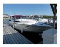
Length 35' 11" 33' 7" LOA Beam 11' 11" Draft 2' 10" 52 Gallons Fuel 172 gallons Water 28 Gallons Waste Weight 10,500#
