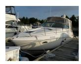
35' 8" 11' 4" L.O.A **Beam** 36"/22" **Draft** 14,100 # Weight (Dry) Water Fuel 168 gallons 50 gallons 6' 6" 47 gallons Waste Headroom
