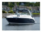
33' 10" 11' 4" LOA **Beam** Draft 36"/22" Fuel 165 Gallons Water 51 Gallons Weight 12,360# Waste 45 Gallons Sleeps Headroom 6' 5" **Deadrise** 18°
