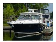
13' 0" LOA 37' 7" (w/pulpit and 30" platform) Beam Draft 3' 0" Fuel 256 Gal Water 38 Gal Waste 20 Gal 15,950# (dry) Weight **Deadrise** 18° (transom)
