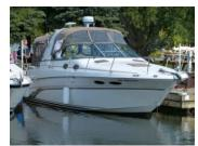
31' 8" 10' 2" Length Beam Draft 37" (25" drives up) Fuel 130 gal. Water 28 gal. Waste 28 gal. 21° Weight 10,500 lbs. Deadrise
