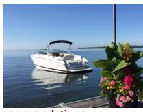
Length 25' 7" LOA 27' 7" (w/platform) Beam 8' 6" Deadrise 21° (at transom) 73 Gallons Draft 37"/ 21" Fuel Waste Weight 5425 lbs 11 Gallons
