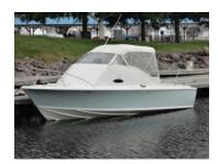
Length25' 11" (with outdrive)Beam9' 11"Max Draft2' 4"Min Draft1' 7"Cockpit Area74 sq ftWeight4,200 lbsFuel110 gallonsSleeps2
